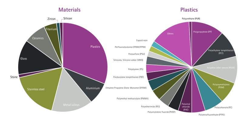
The first diagram shows that plastics represent the majority share of materials treated with the plasma handheld device. Since there is a large variety of plastics, the second diagram shows the different types of plastics that are typically treated with this cold atmospheric pressure plasma.
